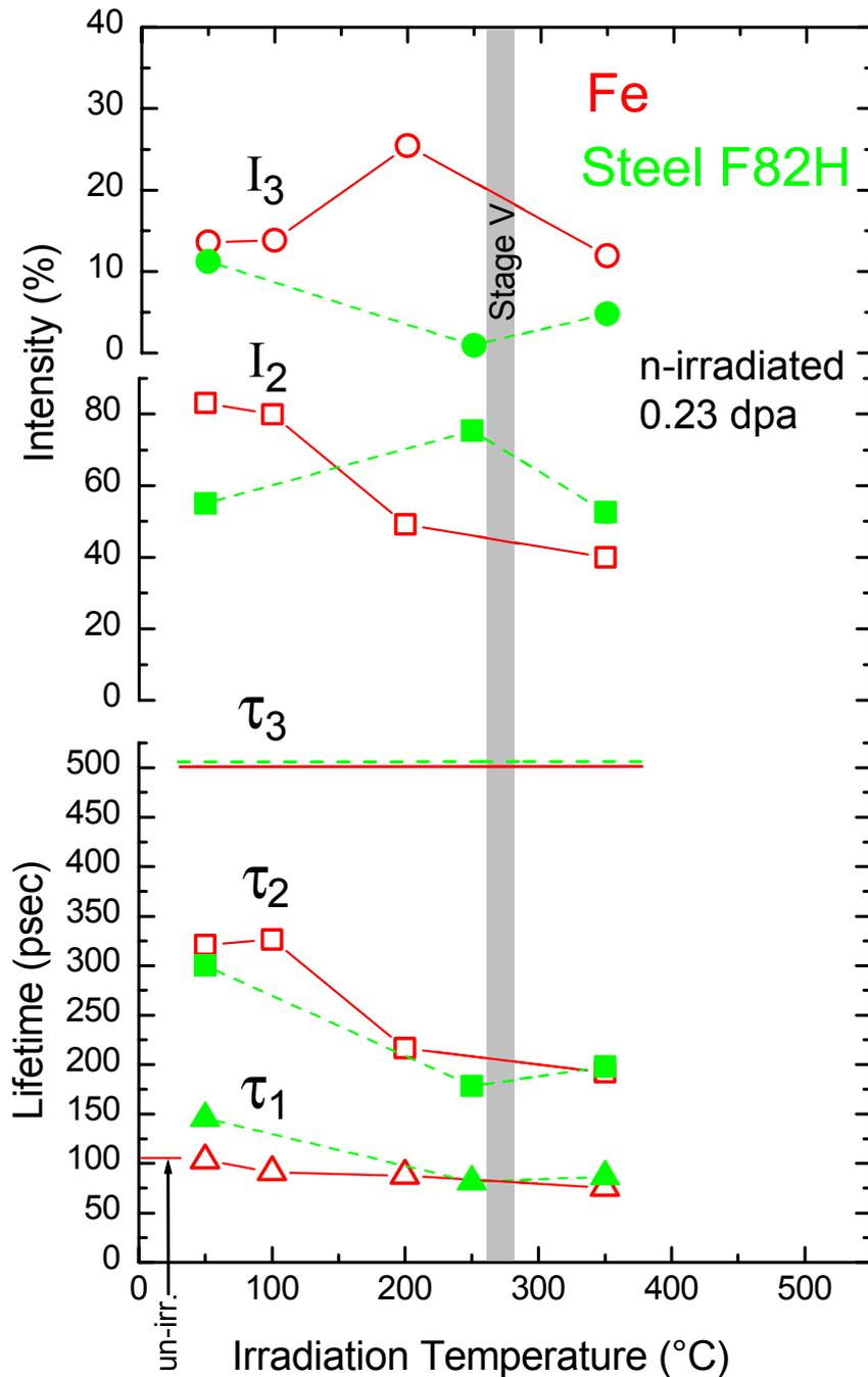
Fig. 3. The three positron lifetimes and the intensities of the two long-lived components ( $I_1 + I_2 + I_3 = 100\%$ ) extracted from the spectra in Figs. 1 and 2 for the neutron irradiated Fe (open symbols connected with full lines) and F82H (closed symbols connected with dashed lines) as functions of irradiation temperature. The longest lifetime,  $\tau_3$ , was fixed at 500 ps in the spectrum analysis. The shaded band indicates the temperature of the recovery stage V.
