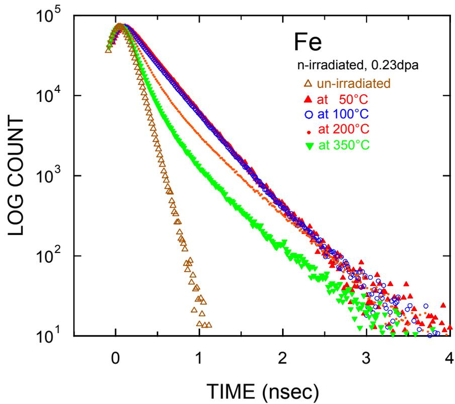
*Fig. 1. Positron lifetime spectra for iron neutron irradiated to 0.23 dpa at different temperatures. The spectrum for un-irradiated iron is shown for comparison. The long lifetimes are indicative of the presence of micro-voids and voids.*
