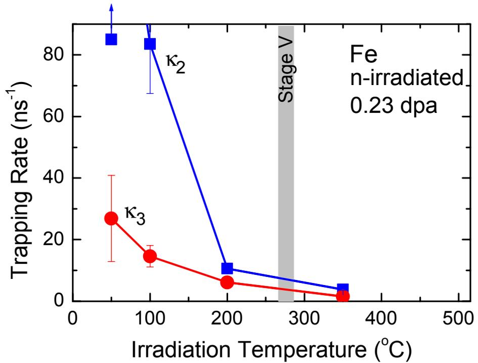
Fig. 4. The positron trapping rates into defects in the neutron irradiated Fe as functions of irradiation temperature, derived from the data in Fig. 3. The circles are for trapping into voids ( $\tau_3 = 500$  ps) and the squares into micro-voids (at 50 and 100°C) or small clusters (at higher temperatures). The indicated error bars are based on the statistical scatter of the data points in the lifetime spectra. The shaded band indicates the temperature of the recovery stage V.
