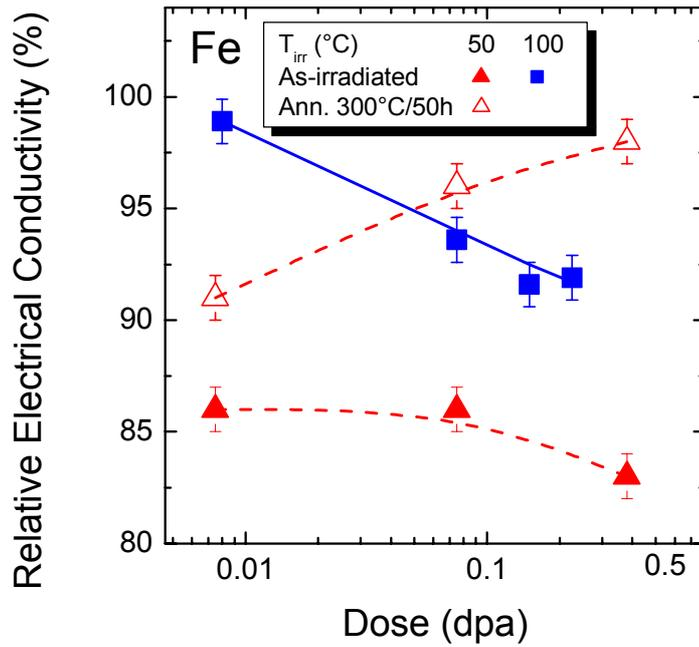
Fig. 7. Electrical conductivity as a function of radiation dose for Fe irradiated at 50°C and at 100°C. Results for the former specimen are shown for the as-irradiated state and after annealing at 300°C for 50 hours. The plot shows the conductivity relative to that for un-irradiated Fe.
