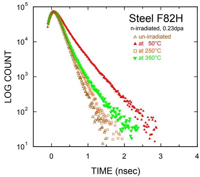
*Fig. 2. Positron lifetime spectra for F82H steel neutron irradiated to 0.23 dpa at different temperatures. The spectrum for un-irradiated steel is shown for comparison. The longest lifetimes are indicative of the presence of micro-voids and voids.*
