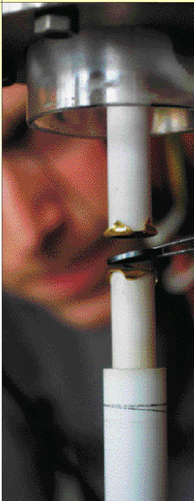
Jens Høgh mounting a ceramic membrane disk to be tested for its oxygen transport properties.
