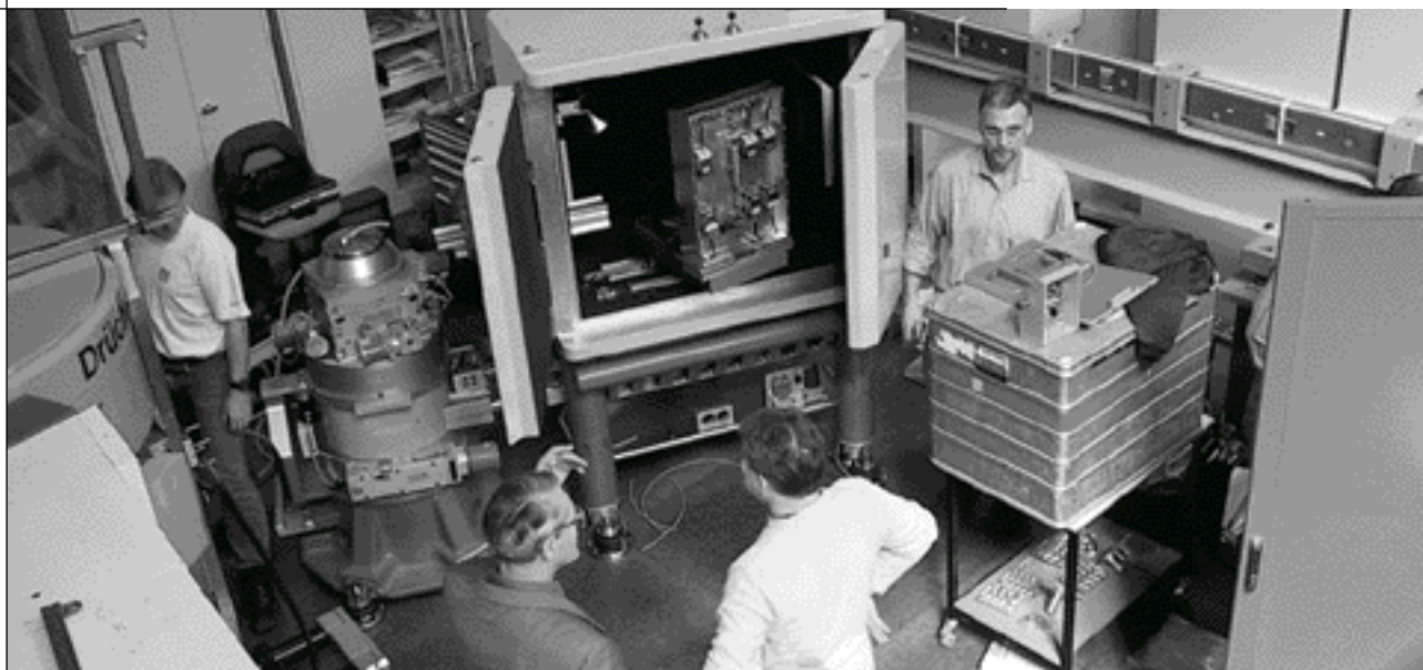
Installation of RITA-II at PSI in May 2001. The spectrometer was moved to PSI in April, and was already taking its first data in June! Shown in the picture are Steen Bang and John Holm from AFM along with some colleagues from PSI. The instrument will be used to study fundamental magnetic properties of materials, including magnetic nanoparticles, superconductors, etc.
