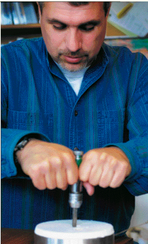
In the supercooled liquid state the amorphous alloy becomes remarkably soft. Nini Pryds is pressing an Mg_{60}Cu_{30}Y_{10} alloy lightly with a tool at approx. 160 °C.
