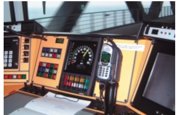
View from the train driver's position crossing the Øresund Bridge. The interface to the current MSR-3 radio is shown on the left and the current GSM-R system is the handset shown to the right of the speed indicator.
