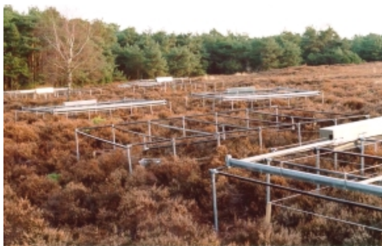
Figure 4 The site Oldebroek in the Netherlands showing the study plots with the scaffolding carrying the curtains to manipulate temperature and water.
