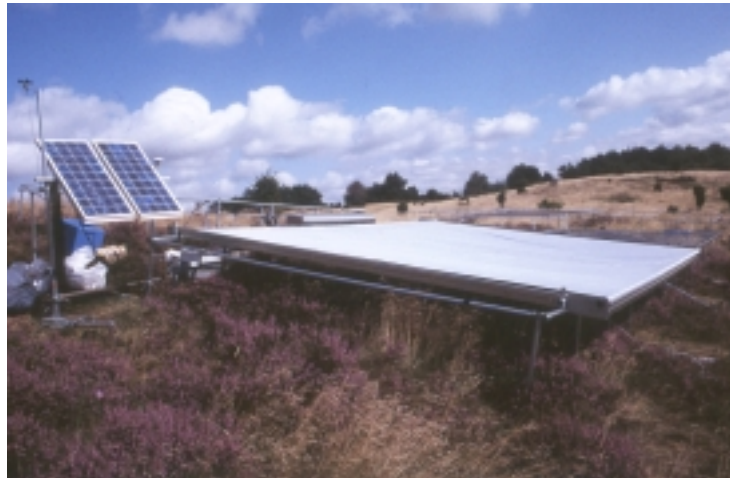
Figure 2 Heating roof covering a heath ecosystem at Mols, Denmark. Power to run the manipulations is supplied by a solar panel.
