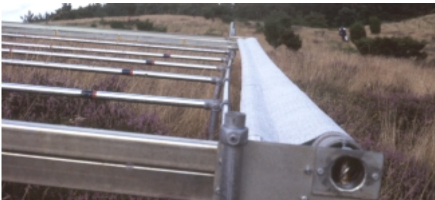
Figure 3 Aluminum curtain used to manipulate temperature. The curtain is rolled up on a beam and are automatically rolled out at night.
