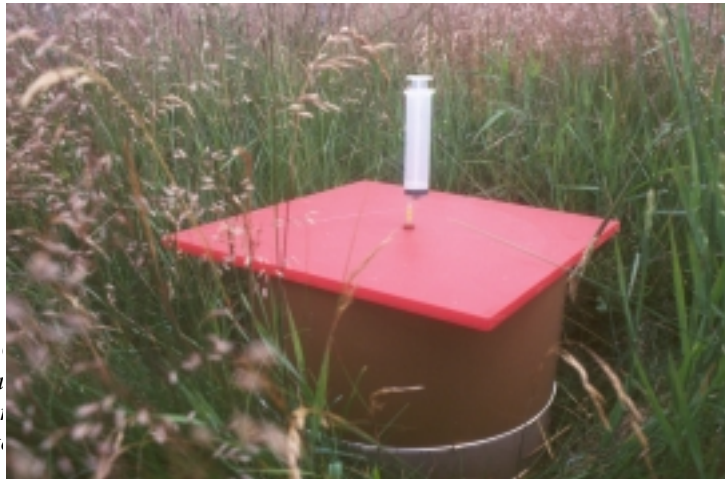
Figure 10 Changes in trace gas fluxes ( \text{N}_2\text{O} and \text{CH}_4 ) in and out of the ecosystem as affected by the treatments are measured in static chambers. The change in trace gas concentration is measured in the chamber after closure.
