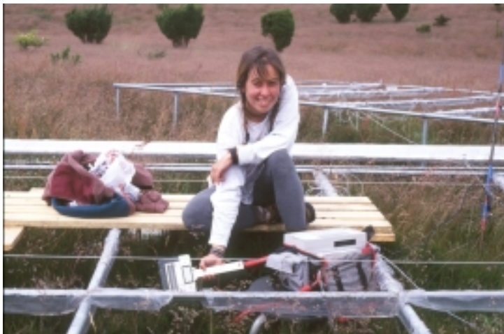
Figure 9 Gas exchange measurements. The changes in photosynthetic activity and respiration are measured by measuring the exchange of CO 2 at the leaf level.
