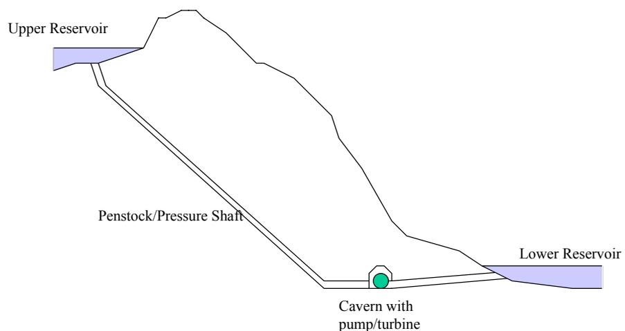
*Figure 2 Principle layout of pumped storage plant*
