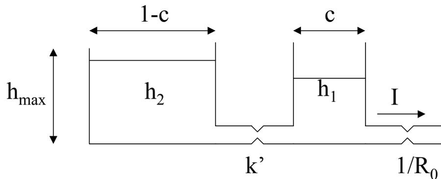
Figure 10 Battery model
