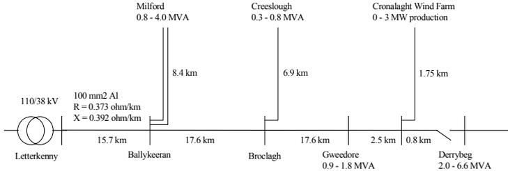
Figure 11 Data for Letterkenny - Derrybeg 38 kV feeder with indication of minimum and maximum loads.
