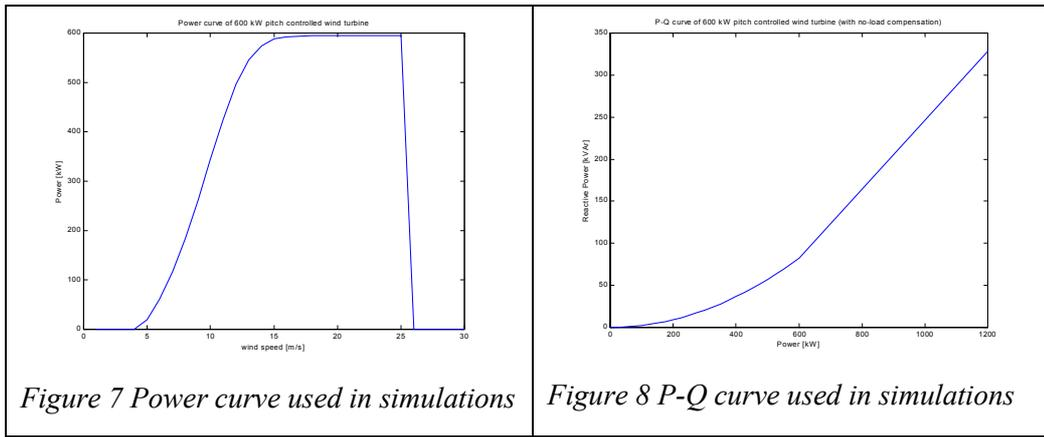
Figure 7 Power curve used in simulations
