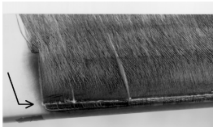
Figure 6.1. Oil flow visualisation on a rotating blade, Re \approx 2.7 \times 10^6 . The arrow points out the trace of the laminar separation bubble, which is the white line at the leading edge. The flow is from bottom to top.
