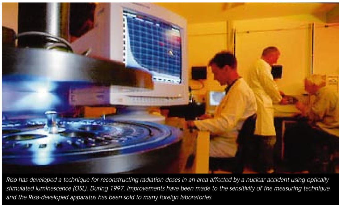
*Risø has developed a technique for reconstructing radiation doses in an area affected by a nuclear accident using optically stimulated luminescence (OSL). During 1997, improvements have been made to the sensitivity of the measuring technique and the Risø-developed apparatus has been sold to many foreign laboratories.*
