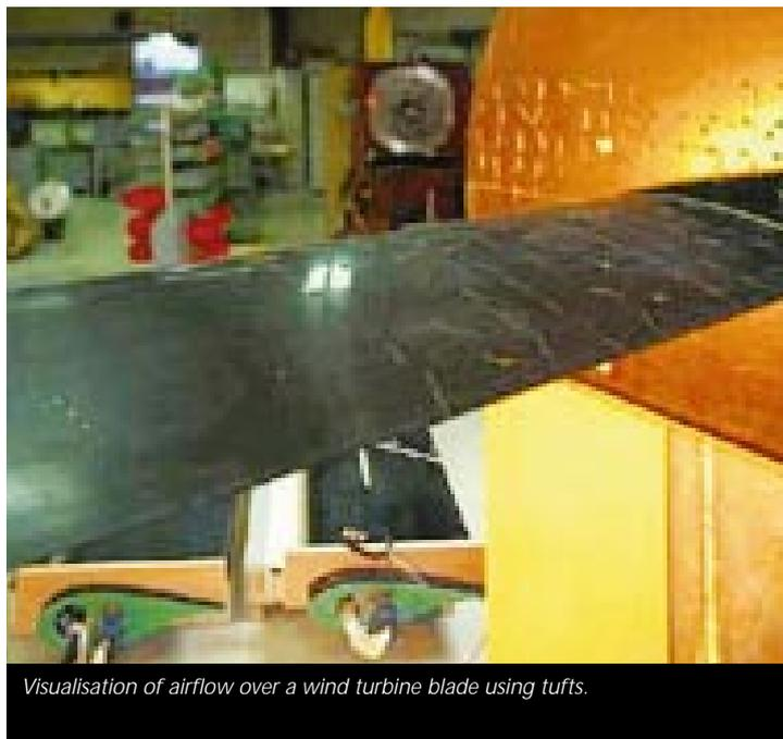
Visualisation of airflow over a wind turbine blade using tufts.
