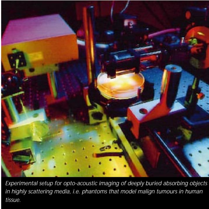
*Experimental setup for opto-acoustic imaging of deeply buried absorbing objects in highly scattering media, i.e. phantoms that model malign tumours in human tissue.*
