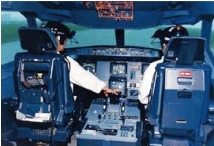
*The Airbus 340 simulator at Aerospatiale, Toulouse, France. The pilots are wearing eye trackers during this experimental study of pilot behaviour during scenarios of abnormal take-offs. Risø was responsible for the experiment and subsequent analyses.*
