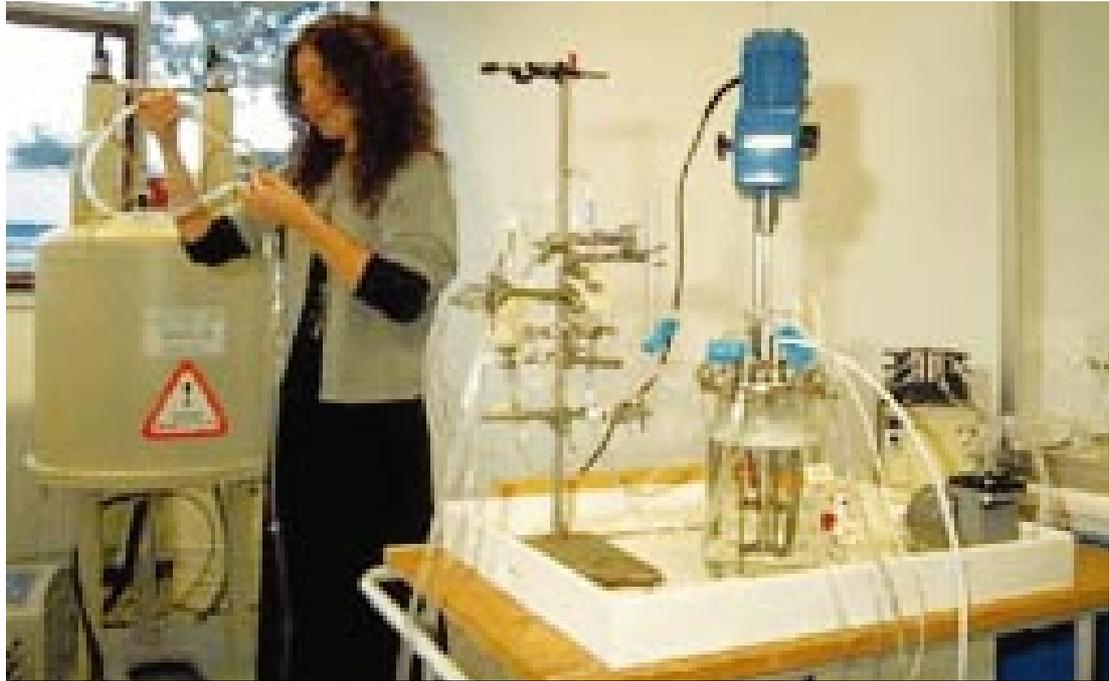
Equipment for NMR spectroscopic studies of nitrogen fixation in living plant-microbe symbioses. The research is being undertaken by the Centre for Plant-Microbe Symbioses supported by the Danish National Research Foundation.
