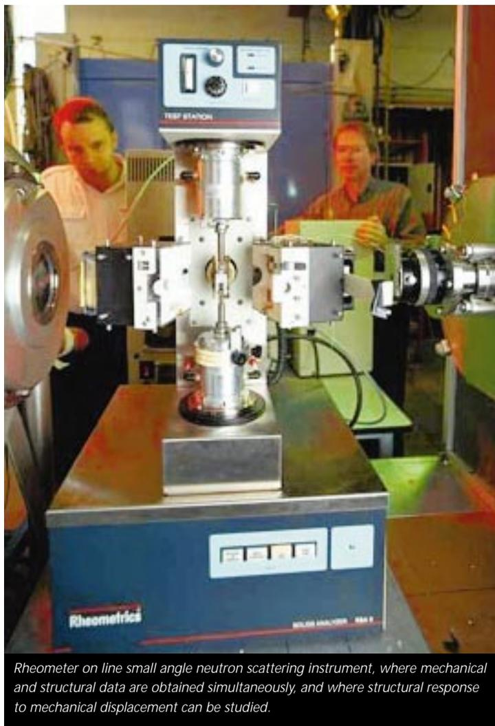
*Rheometer on line small angle neutron scattering instrument, where mechanical and structural data are obtained simultaneously, and where structural response to mechanical displacement can be studied.*
