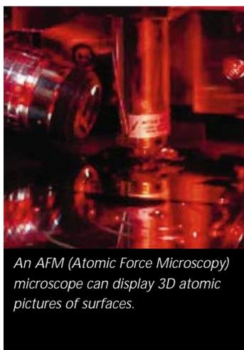
*An AFM (Atomic Force Microscopy) microscope can display 3D atomic pictures of surfaces.*
