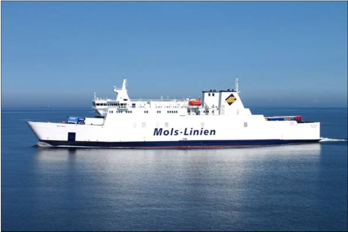
Fig. 1 1200 lane metre Ro-Ro passenger ship (Mette Mols) for 600 passengers
