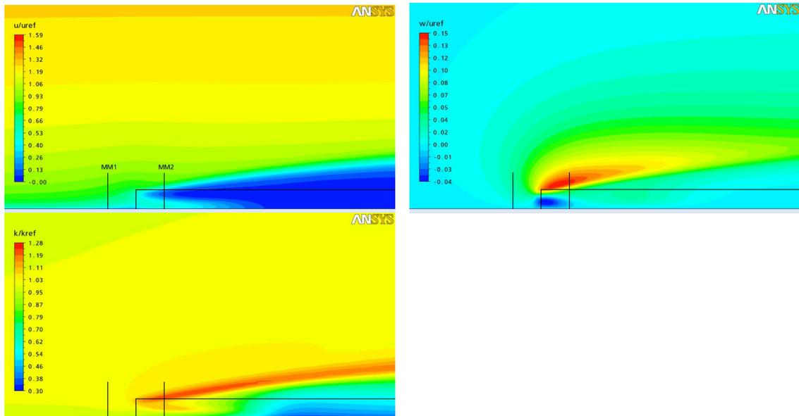
**Figure 5 – CFX contour plots of  $u/u_{ref}$  (top left),  $w/u_{ref}$  (top right) and  $k/k_{ref}$  (bottom left) for summer conditions. Met mast positions and location of the forest are included. Wind direction is from left to right.**
