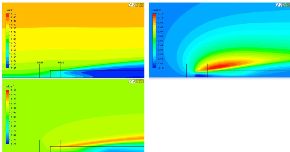
**Figure 6 - CFX contour plots of  $u/u_{ref}$  (top left),  $w/u_{ref}$  (top right) and  $k/k_{ref}$  (bottom left) for winter conditions. Met mast positions and location of the forest are included. Wind direction is from left to right.**
