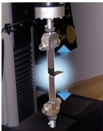
Figure 1: Apparatus to determine the peel strength.
