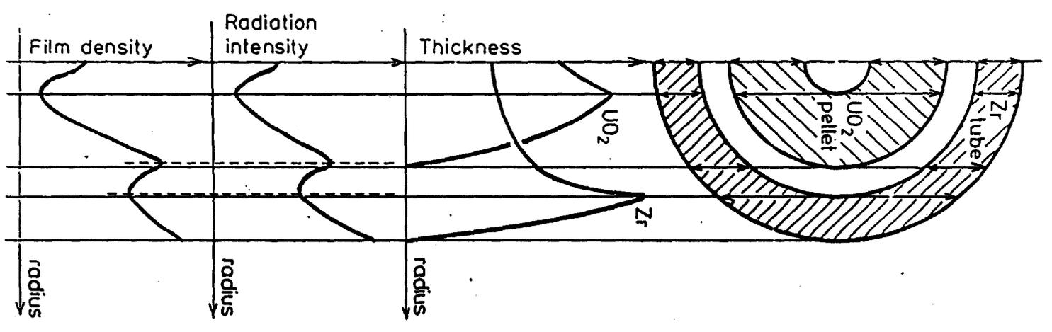
Fig. 6. Thickness, radiation intensity and film density
