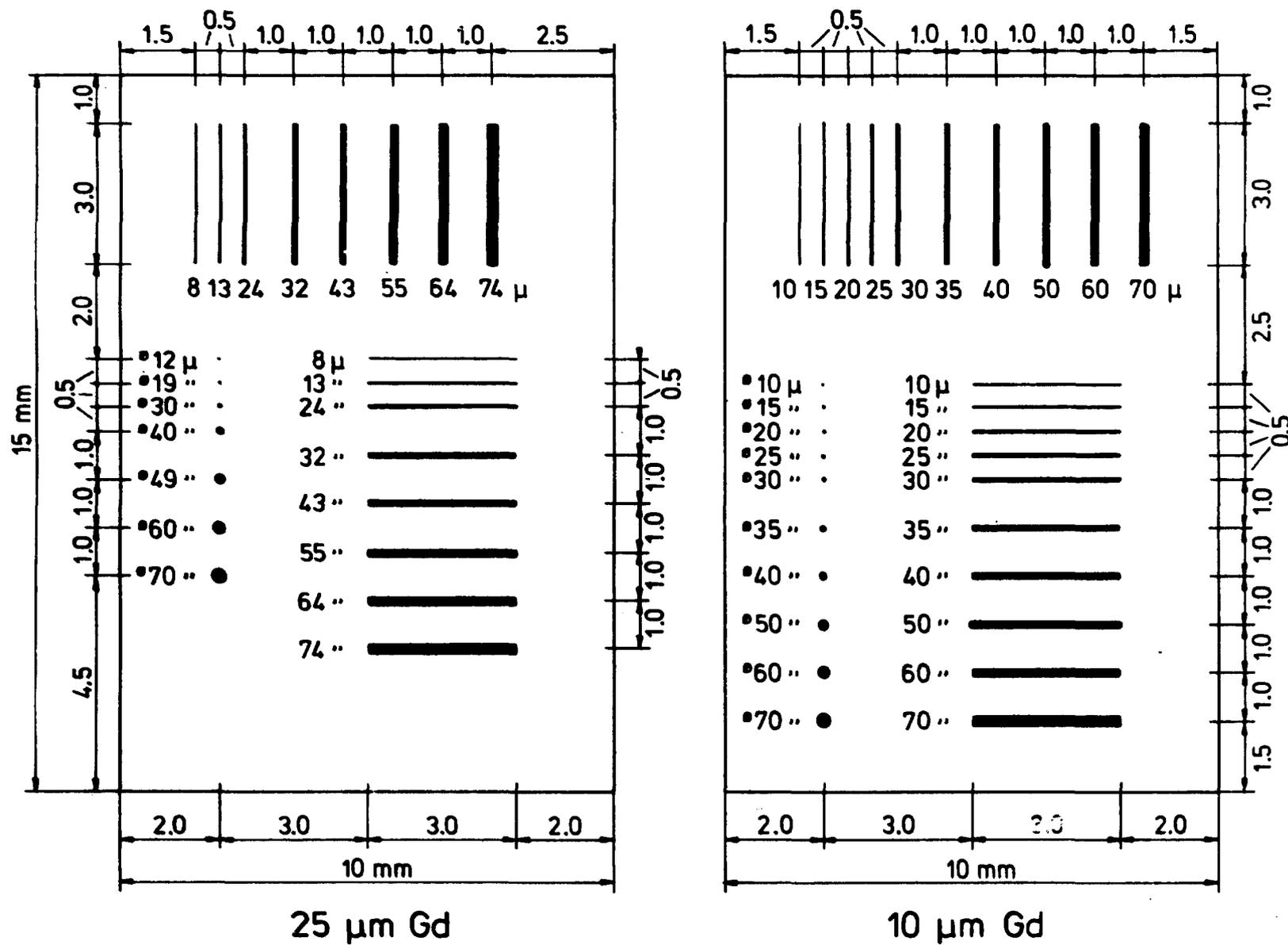
Fig. 4. AFNOR IQI. Fabricated (left). Designed (right).
