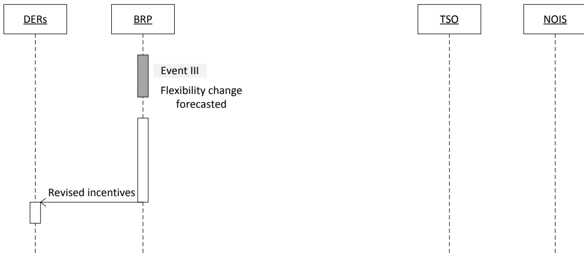
Figure 8 Alternative sequence showing communication in the Manual Regulating Power Market when one or more DERs experience small changes in their flexibility which does not require changing bids from the BRP, under indirect control architecture.
