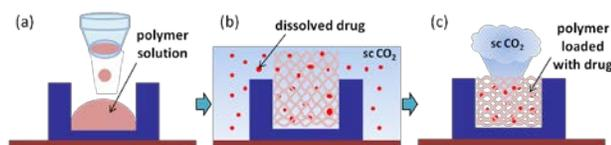
Figure 1 Drug loading process: (a) Inkjet printing of PVP solution; (b) scCO<sub>2</sub> impregnation: pressurization and polymer swelling, (c) depressurization and de-swelling.
