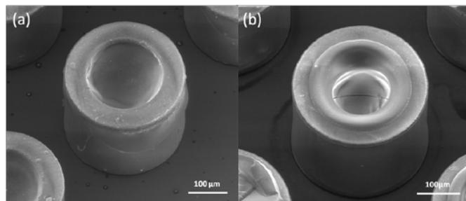
Figure 3 SEM pictures of microcontainer impregnated at a CO<sub>2</sub> pressure of 100 bar (a) and 200 bar (b).
