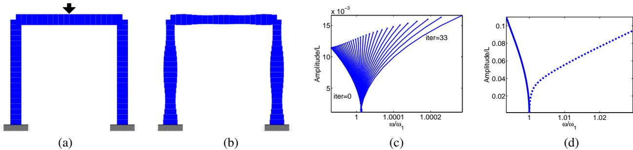
Figure 1: (a) Optimization problem, (b) optimized design, (c) evolution of backbone during iterations and (d) comparison of initial backbone and optimized backbone at larger load. solid line: initial design; dashed line: optimized design.
