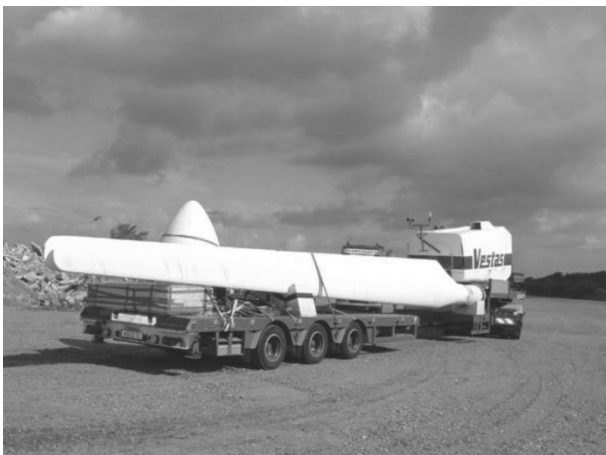
Fig. 6 Transport of rather small EoL WT blades by Green-Ener-Tech Denmark [11]
