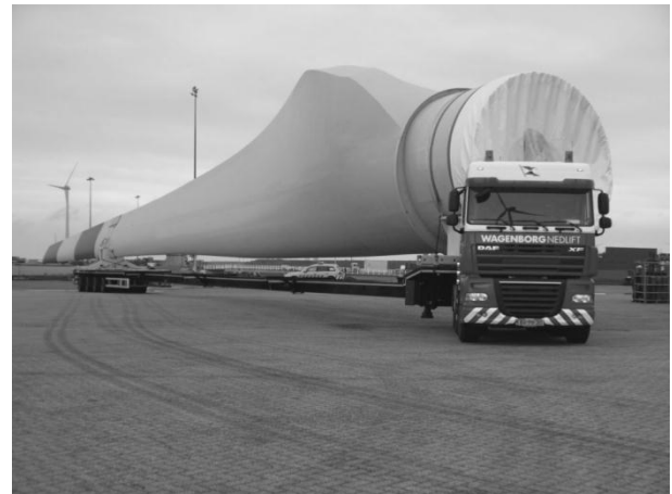
Fig. 7 Transport of a 59 m long blade [17]
