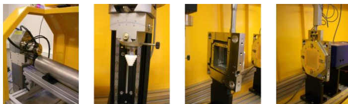
Figure 2: Experimental set-up at Niels Bohr Institute. From left to right: X-ray source and source grating (G0), rotary table and step cylinder, phase grating (G1), and analyzer absorption grating (G2) followed by a detector.
