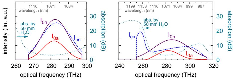
Fig. 3. The shape of a state-of-the-art broadband spectrum (left,  $\Delta\nu = 30$  THz) changes only slightly due to water absorption, and compensation would require only a minor redistribution of power from the center to the edges. An ultra-broadband spectrum (right,  $\Delta\nu = 60$  THz) gets strongly attenuated below 265 THz, and a large fraction of the total power is required to compensate for this.  $I_{0n}$  and  $I_{cn}$  are normalized to unity power.
