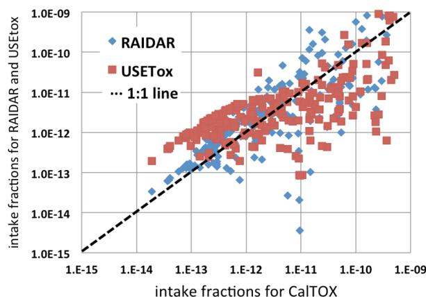
Figure 1: intake fraction comparisons due to emission to fresh water from CalTOX, RAIDAR, and USEtox models
