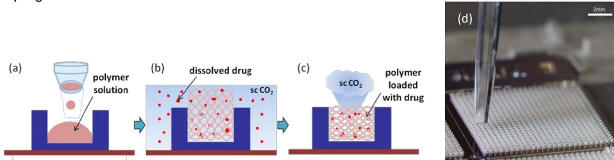
Fig. 1: Drug loading process: (a) Inkjet printing of PVP solution; (b)  $scCO_2$  impregnation: pressurization and polymer swelling, (c) depressurization and de-swelling. (d) Silicon slide placed on the microspotter tray and dispensing pipette. Each slide contains 625 containers.
