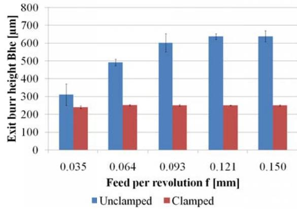
Fig.8. Effect of clamping on exit burr height.
