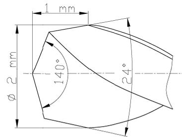
Fig.9. Profile of double cone point drill A.
