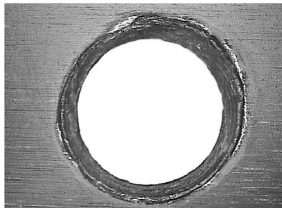
Fig.7. Hole entry defect.
