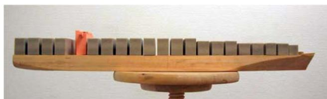
**Figure 6 - Wind tunnel model with fully stacked deck.**
