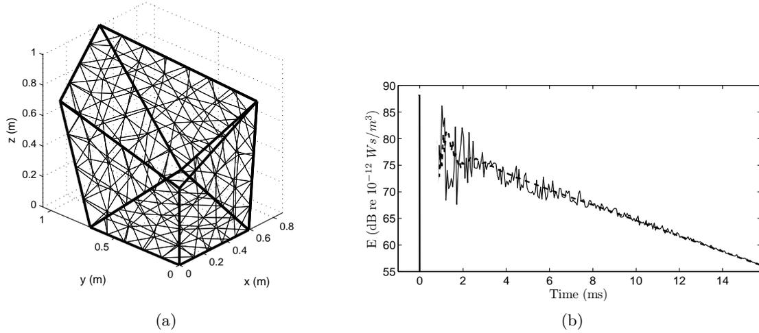
Figure 3: (a): A 7-wall polyhedral room meshed with  $N=276$  triangular elements. Source:  $Q = (0.3, 0.2, 0.2)$  m. Receiver:  $P = (0.4, 0.7, 0.5)$  m.. (b): Reflectograms at the receiver in the room. Coefficients from Table 1. ---: Case 1. —: Case 2.
