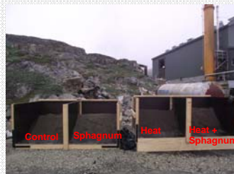
Third approach set-up: Boxes with oil-contaminated soil and different additions. The addition of sphagnum includes both sphagnum moss and chalk.
