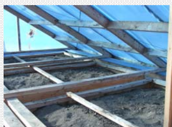
First approach set-up. The excavated soil was placed in the blue "tent" (top picture) in different wooden boxes (bottom picture). Heat was generated by solar energy.
