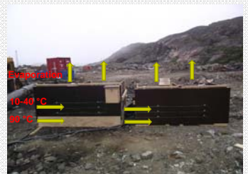
Third approach set-up: The heating set-up and temperature measurement system.
