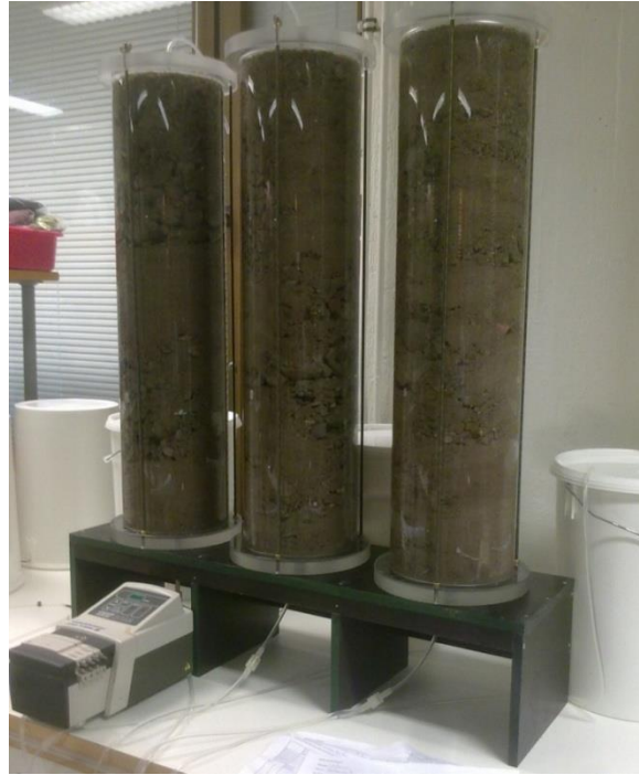
Figure 8. Leaching test performed with coarse materials implies use of large columns and long test duration. Large columns are impractical and demanding, therefore a limit for maximum particle size of test materials have been set.
