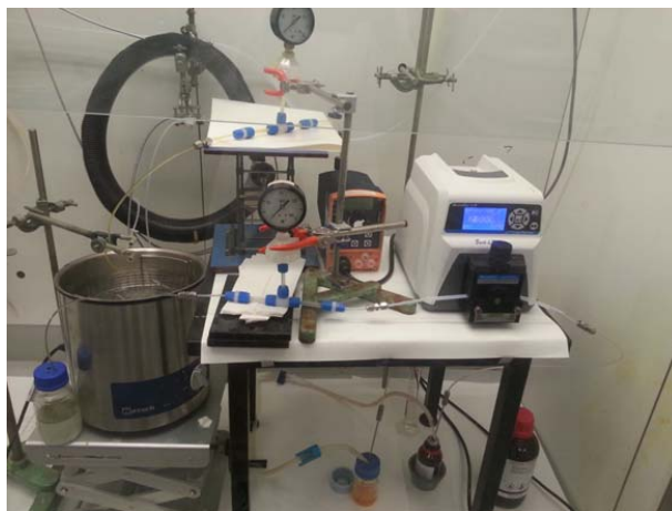
Figure 8.8 Experimental setup for performing the chemical reaction between 2-bromophenyl hypochlorothioite and phenylmagnesium bromide in continuous mode. a) Process flow sheet including: T1, T2, T3 – tanks; P1 and P2 – pump; M – manometers. b) Photo of the setup
